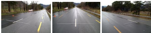
Left middle and right image with a 5m surveying rod as scale information
