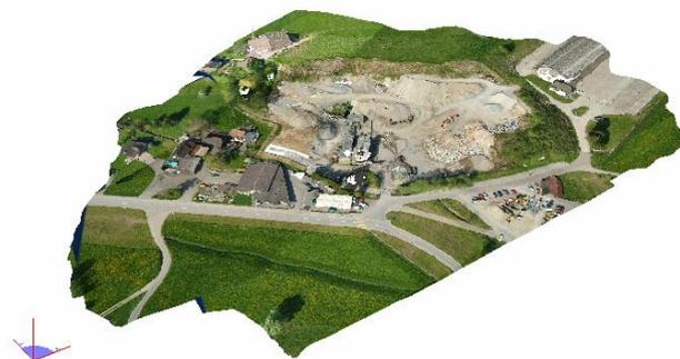
In aerial photogrammetry like in this example we can generate a contour map of the area very easily using the built in functions from the ELCOVISION 10 AutoCAD Tools with a few mouse clicks:
