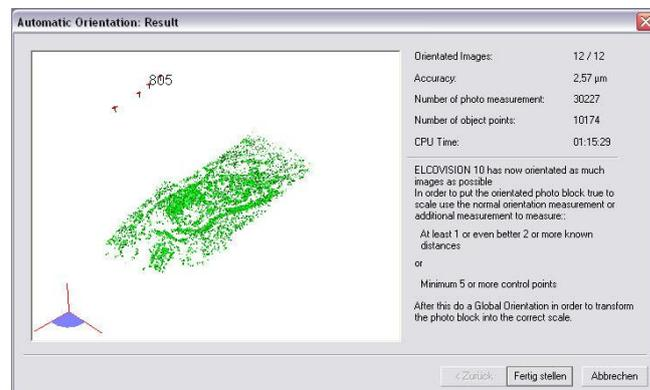
Now it is time for the first and only manual step in the automatic orientation process. The operator should define a suitable system of coordinates. This could be done by measuring at least one known distance or by measuring at least 4 control points.
