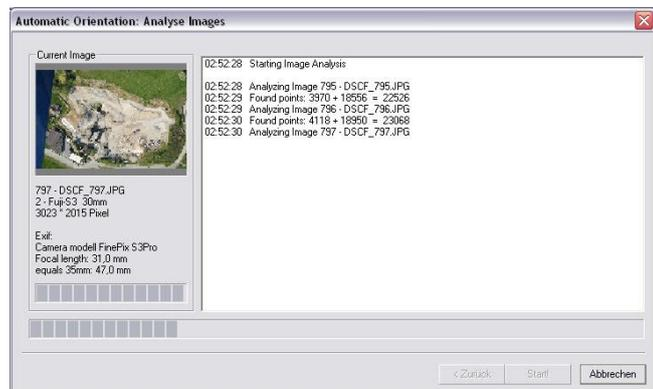
In the next step ELCOVISION 10 uses this featured points found in the first step and runs the automatic orientation using the traditional relative, absolute and global orientation approach.
