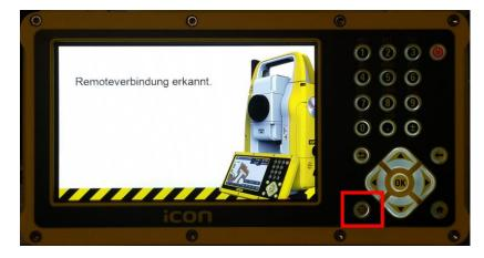
In this mode, measurements can now be done normally with the theodolite measurement button (crosshairs button at the bottom left of the cursor buttons). Note that all other buttons on the instrument have no function anymore.
