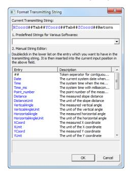
THEO online simulates normal keyboard input of a user. Therefore nearly all applications can be fed with measurements of a total station. The measurements can be formatted in virtually all possible ways, so that nearly all applications can benefit from THEO online.
