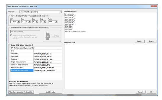
In the small THEO online window and in the configuration dialog above a button [GeoCOM online] appears. With this button the measuring mode of the theodolite can be switched on and off.
