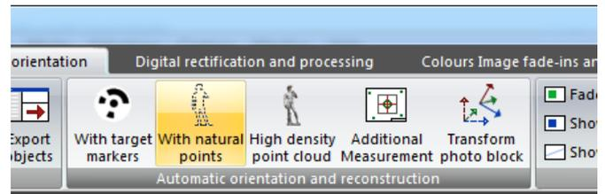
**ELCOVISION 10** orients and optionally calibrates all cameras and calculates a high density point cloud of the object.
