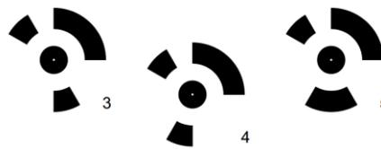
These targets are measured fully automatically with a high subpixel accuracy by **ELCOVISION 10** and thus, when using high-quality cameras, achieve high accuracies in the 0.02mm range even on large objects such as bridges. This allows very accurate deformation measurements to be carried out.
