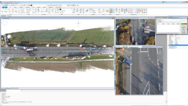
Here you can also import the point clouds or Orthophotos into the CAD drawing with a few mouse clicks and continue working there. With the help of further image measurement functions you can generate further evaluations such as contour maps, profile sections or simply dimension an Orthophoto.
